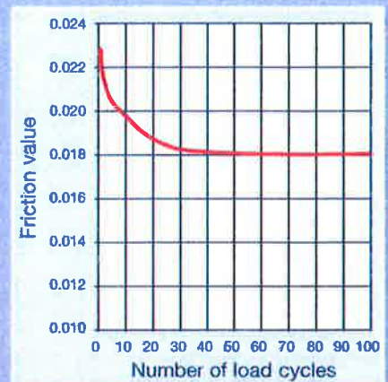
Figure 8: Friction values for Ciparall® Sliding Bearing, values as a function of load cycle number after stop times are terminated
