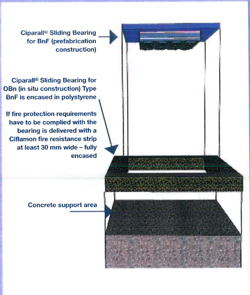
Figure 10. Installation principle of type BnF or OBn on a concrete column
